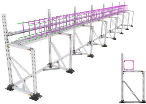
Bench Setup 8.4 x 0.6m (90cm working height) 28 x 2' (3' working height)
